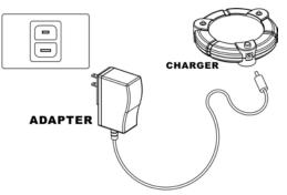
**Step 2**: When the charger is powered, charger power LED will illuminate to show it is on.
